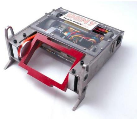
Drum-The drum is a bladed robot with a cylindrical blade spinning on a horizontal axis. The blade is commonly a tube or pipe with several "teeth" installed to cut at the opponent.
