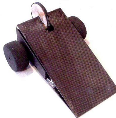
Rammer- A ramming robot uses its body to push and smash into other robots either inflicting direct damage, trapping, or causing the opponent to self-inflict damage (a blade consequently hitting into a wall causing damage). For inexperienced teams a design such as the rammer bot is fairly simple to construct due to its basic design and few components.
