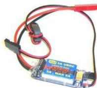
**BALANCER** - A battery balancer or battery regulator is a device in a battery pack that performs battery balancing, they regulate the rate that each cell in a pack is charged. A balancer may be added to a battery pack when charging. They come in different forms a “blinky” is pictured
