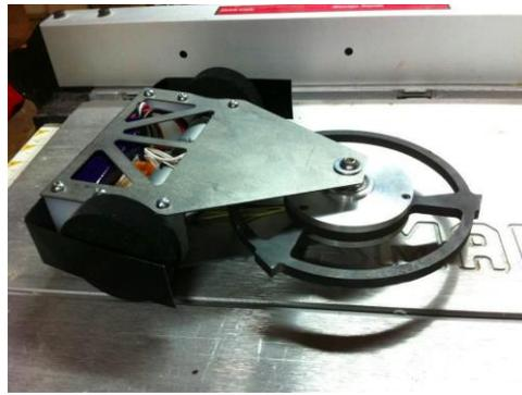
Eggbeater- The eggbeater is a bladed robot with a flat blade spinning on a horizontal axis. The blade is commonly a rectangle but many other shapes have been used.
