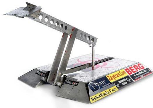
Hammer/ Thwackbot- A thwackbot may use a hammer, ax, pick or whiplike hammer to strike their opponent. There are variations of this type where the striker is either on a horizontal plane or vertical. The striker may be activated using an actuator or simply by spinning the robot.
