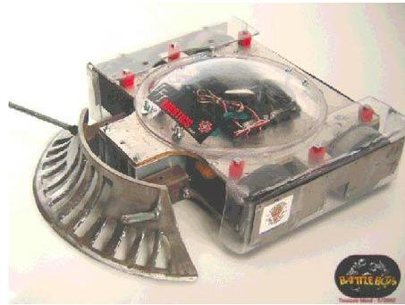
Flipper/ launcher- A flipper robot may use a spatula type lifter or other to intentionally lift their opponent from the arena floor to incapacitate them.
