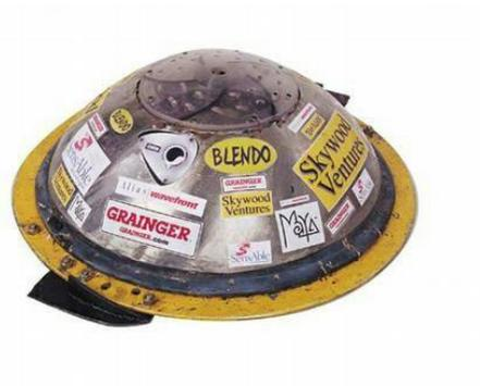
Horizontal-blade- Robots using a horizontal blades have a blade traveling on a horizontal plane, they function similarly to the spinner except that only a blade spins on a vertical axis under, over, or around the robot body. Blades vary from saw blades to bars of metal similar to a lawn mower.
